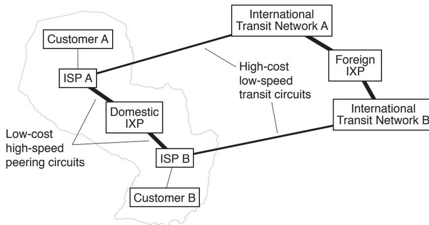
Figure 1: Two ISPs connected through a domestic IXP and via international transit networks
