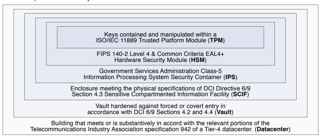
Together, the TPM, HSM, IPS, SCIF, Vault, and datacenter comprise six concentric layers of physical security, each successively harder to compromise than the last, to provide tamper resistance and tamper evidence protecting the key material and zone-signing process at each location.
