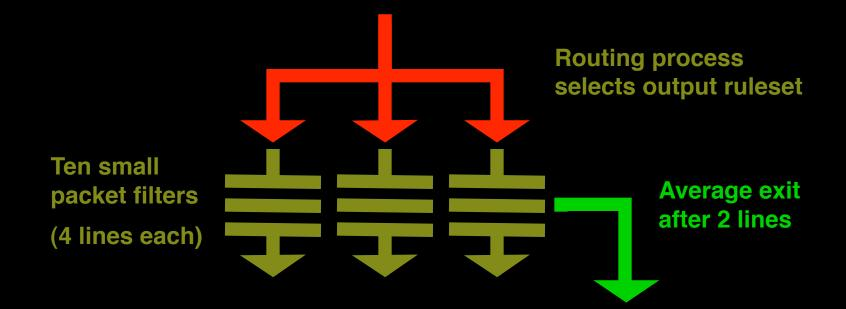
Routing is cheap, ruleset processing is expensive. Use the router for what it's good at.
