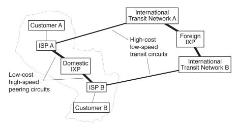
Figure 1: Two ISPs connected through a domestic IXP and via international transit networks
